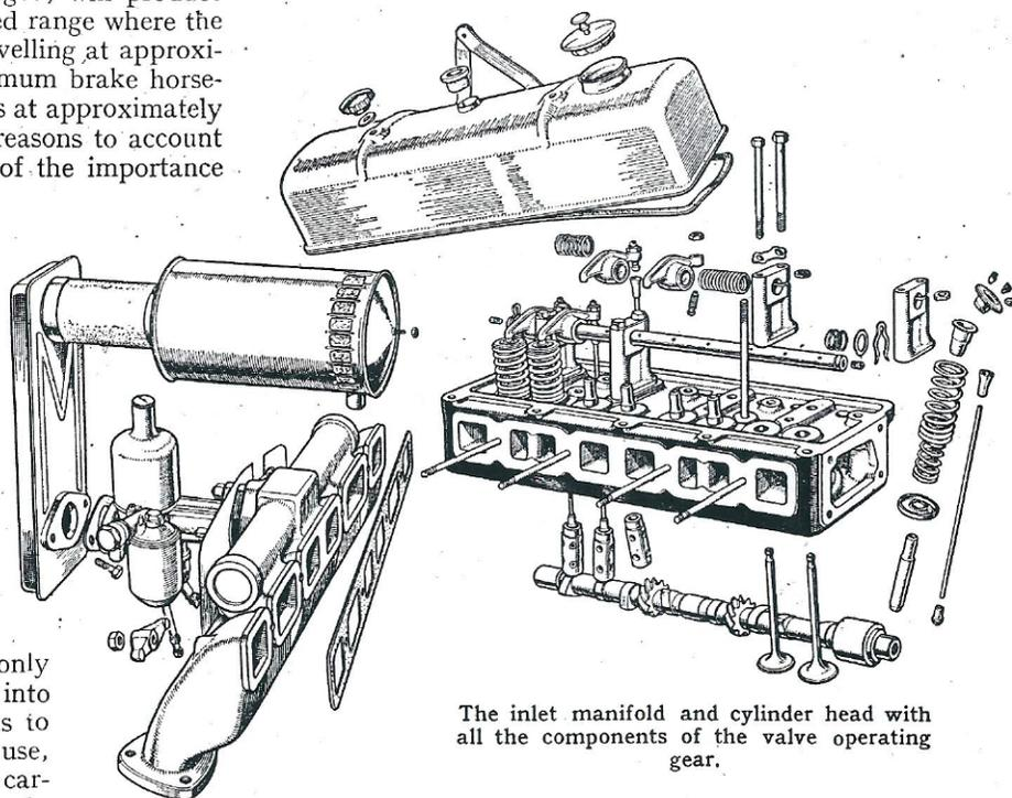
The inlet manifold and cylinder head with all the components of the valve operating gear.
