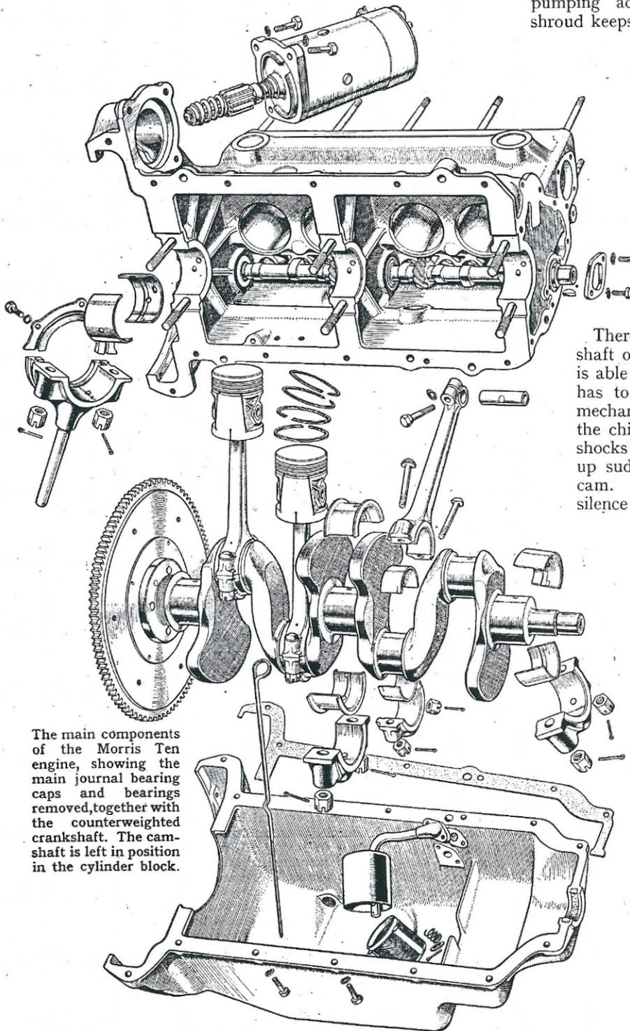
The main components of the Morris Ten engine, showing the main journal bearing caps and bearings removed, together with the counterweighted crankshaft. The camshaft is left in position in the cylinder block.
