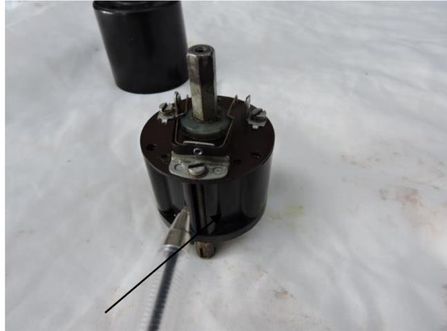
5. Each screw acts as a conductor between the contact plate and the brass terminals on the base. The lower screw in the photo passes through the common terminal for the two moving contacts and connects to the base terminal marked F. When assembling takes place this is the correct position for the contact plate.
