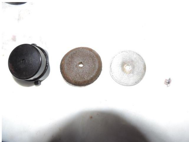
9. Clean all parts as necessary ensuring old grease is removed.
