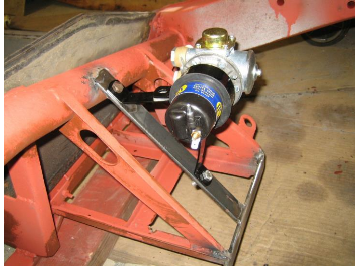
Jig 6: MGB petrol pump on disused battery carrier.
