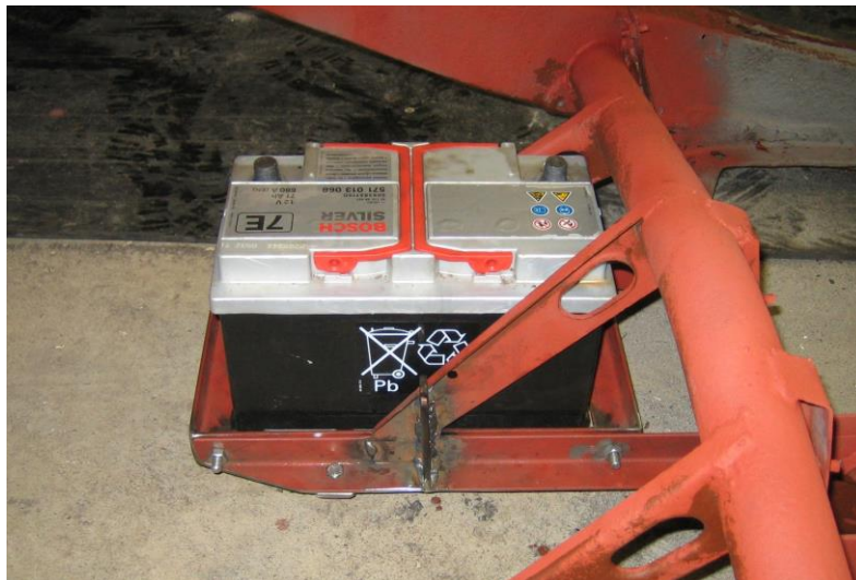
Jig 7: Larger battery mounted on its own pivoting cradle.
