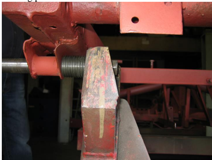
Jig 4: Rear spring rear mounting points.
