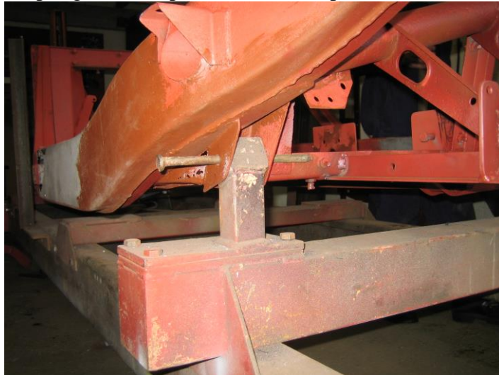
Jig 4: Rear spring rear mounting points.
