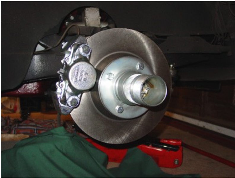
All items bolted in place. Check that the disc runs central in the calliper slot (may need to shim).
