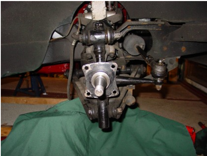
Stripped down to the basic MGA front axle
