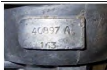
40897 is the service number for the 25D4 used in early MGB's, 163 is the date code for 1 st week of 1963
