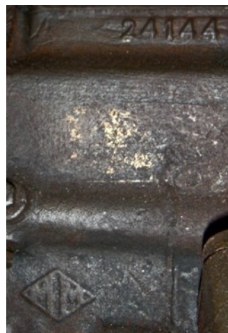
24144 XPJM block casting number
