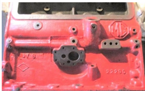
22290 block with date code, plain diamond & MG logos. Photo by Alasdair Enticknap
