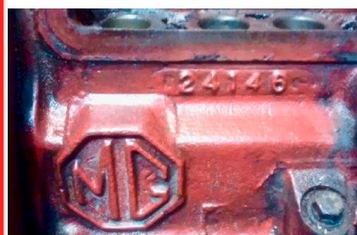
24146 block casting number Photo: Mark Tullett
