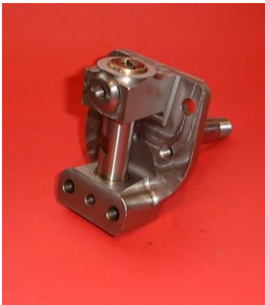
Fig 6: The stub axle with bushes reamed and king pin fitted
