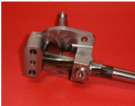
Fig 4 Reaming the first new bush using the remaining old bush as a guide.
