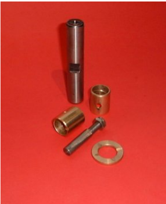
Fig 1: King-pin components. A king-pin set for one wheel comprises the king-pin, two bushes, a thrust washer and a cotter pin. The cotter pin supplied here is not like the original. Note the head of the cotter pin provides a steering end-stop in conjunction with a special bolt that fixes to the back of the stub axle.
