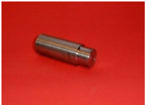
Fig 2: A tool to push out the old king-pin bushes and insert new ones.
