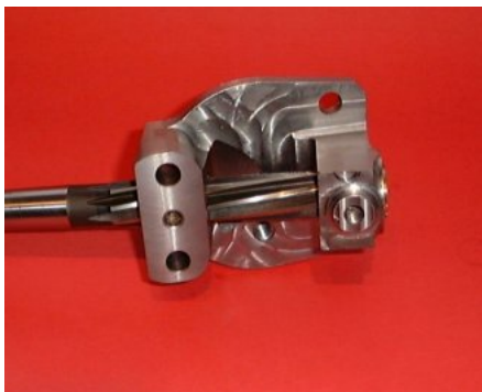
Fig 5: Reaming the second new bush using the other new bush as a guide.
