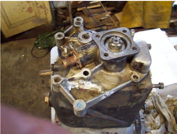
The job in hand – to reinforce the fractured casting.
