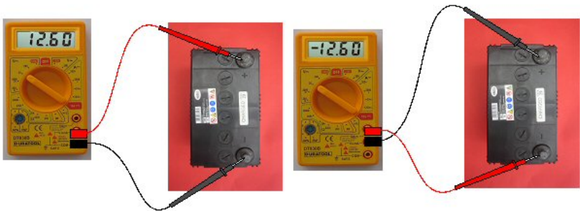
Fig 2 Correctly and Incorrectly Connected Multimeter.
