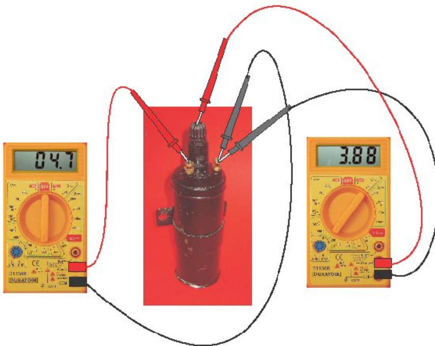
Fig 3 Typical Resistance Readings for a 'Good' Coil. (Primary 4.7 Ohms, Secondary 3880 Ohms)
