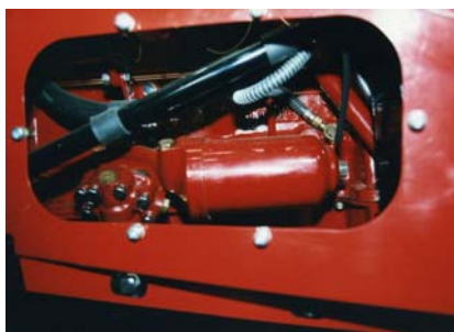
Photos showing heater hoses and fit within the dash panel 'H' frame
