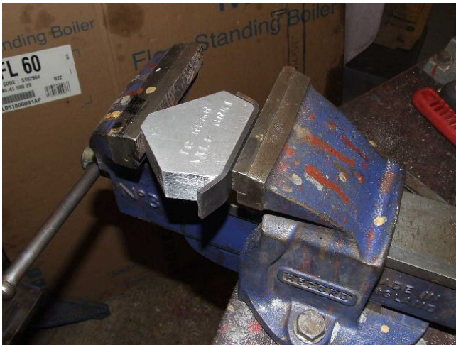
Figure 4 shows the strip of 1 inch wide by 1/8 inch mild steel held against a bending former by the vice jaws. The ends of the steel strip can then be belaboured around the bending former. (Pass me the bigger hammer). Figure 4 (left)
