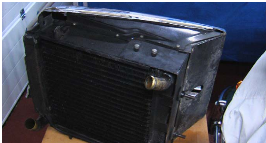
Radiator and shell all in one removed as per Workshop manual.
