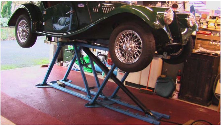
The Autec Electro Hydraulic Car Lift purchased by Dennis Barker (this was put to good use when removing the radiator from the car).
