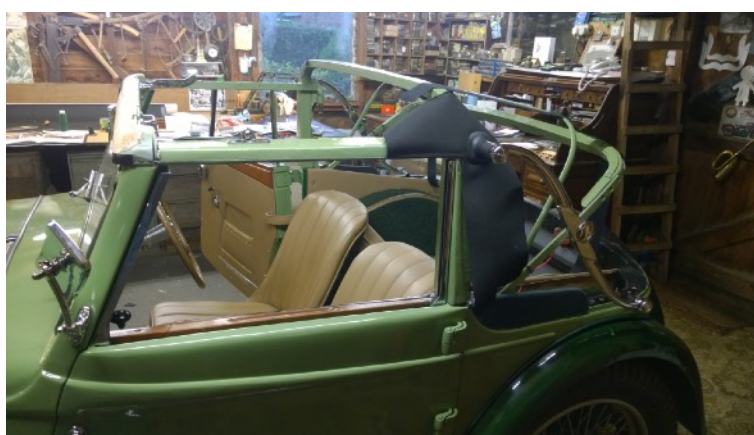
Setting up the hood bows and tension wires for the hood prior to cutting out the fabric.
