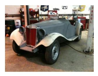
Most of the ash frame was in pretty good nick and had been retained, but two or three parts were not worth bothering with. The floor was completely shot – and was replaced with one piece of heavy-duty marine ply – a much better job than the rotting 'floor boards'.
