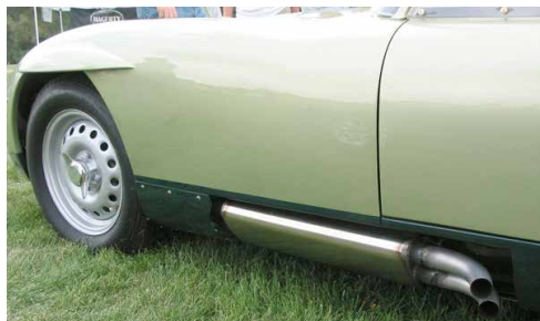
Custom stainless steel muffler built to the original MG engineering drawings.
