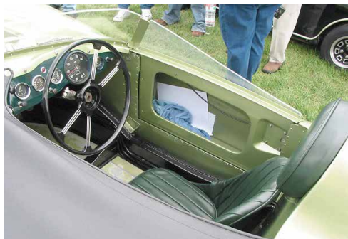
EX186 is a well-crafted car. The custom aluminum doors feature special aluminum hinges, but they utilize standard MGA latches. The doors fit properly, and open and close quite neatly.
