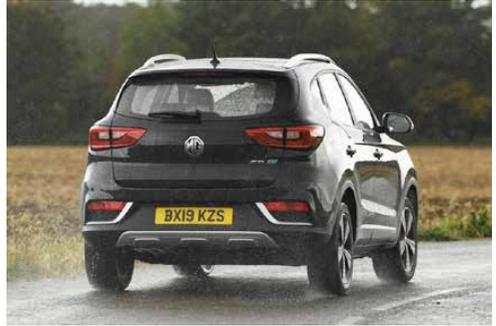
It sprinted from 0-60mph in 7.4 seconds, 0.4 seconds faster than the Leaf, but by 60mph the MG's urgency tails off (its top speed is only 87mph). Acceleration from lower speeds is more important to more people, and in this instance, the ZS managed 30-50mph in 2.7 seconds, compared to 2.8 seconds in the Leaf, so there's little to split them. This acceleration is what makes smaller EVs like these easy and fun to drive in urban areas.
