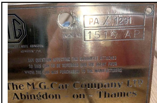
Original guarantee plate PA 1291. Note the etched PA/1291 and the closeness of the numbers
