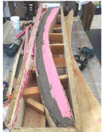
Fig 13 Donor rail held in place with modelling clay, one side poured
