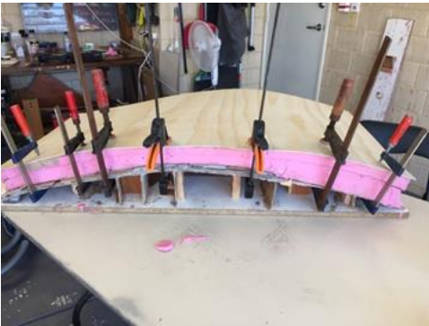
Fig 16 Ply and clamps save expensive rubber Fig 17 pouring second side
