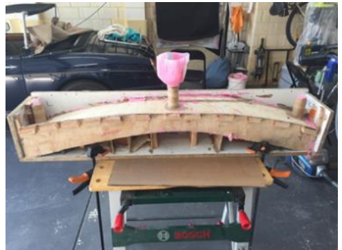
Fig 16 Ply and clamps save expensive rubber Fig 17 pouring second side
