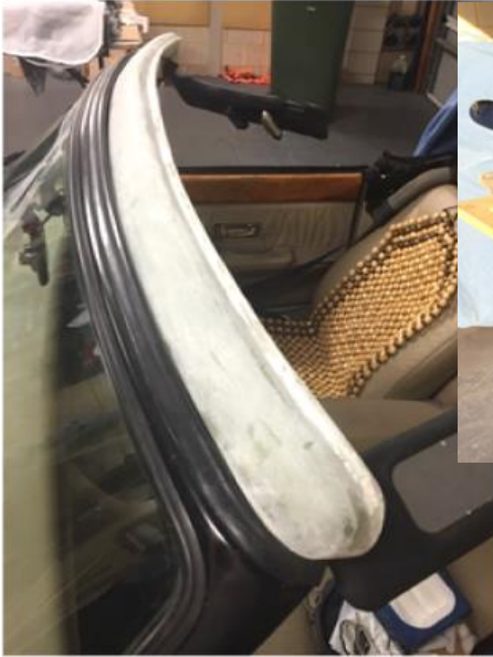
Fig26 (left) trimmed halves glued together
