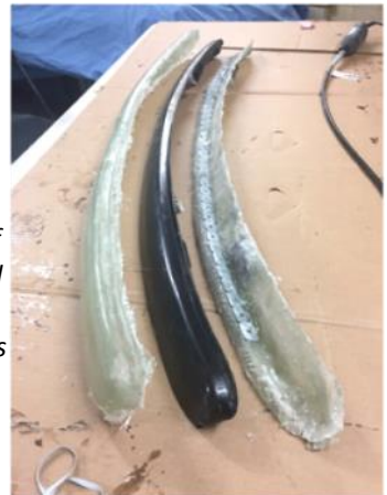
Fig 24 (left) first a gel coat, then three layers of fiberglass cloth
