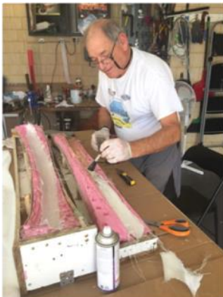
Fig 24 (left) first a gel coat, then three layers of fiberglass cloth
