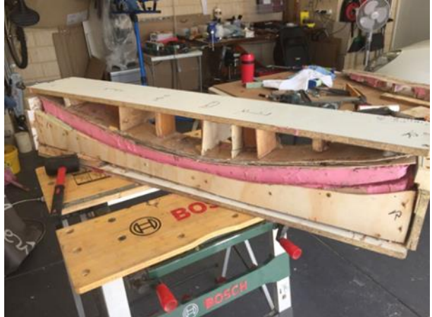
Fig 22/23 (below) mould box converted as support buck to prevent flexure of rubber during fibreglassing
