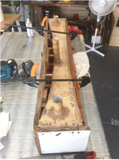
Fig 14 (left) cardboard tubes to pour silicone
