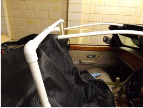
Fig 6 Mk 1 prototype PVC pipe frame
