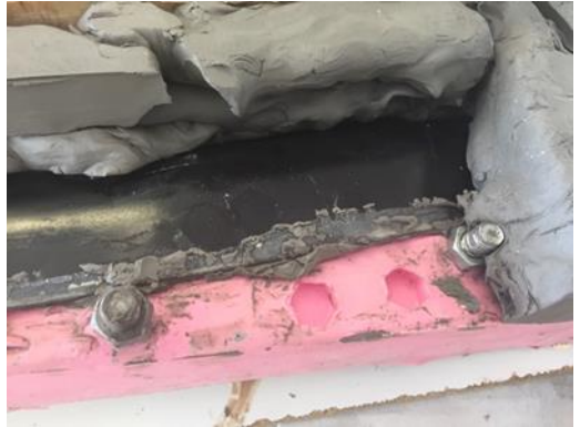
Fig 15 (below) showing bolts to create index points for mould halves
