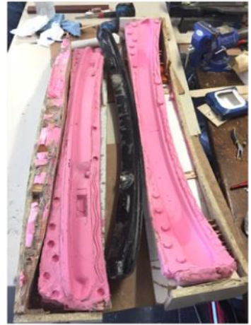
Fig 22/23 (below) mould box converted as support buck to prevent flexure of rubber during fibreglassing
