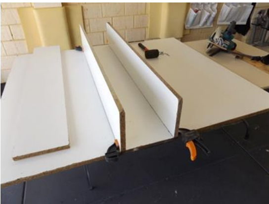
Fig 12 Mould box 18mm laminated particle board
