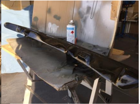
Fig26 (left) trimmed halves glued together
