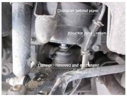
Wheel removed and suspension exposed
