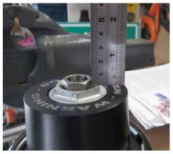
Screw the adjuster into the new spring unit leaving just enough sticking out to get a spanner onto the flats.
