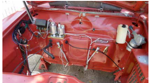
Engine bay, wiring and hydraulics fitted.
