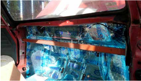
New dash rail fitted.
