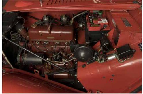
carburettor, single fuel pump and standard-ratio 4-speed gear box).
