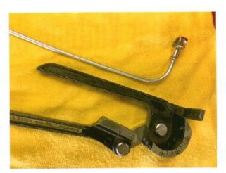
when making a full 90-degree bend, as it may want to collapse. Be sure to check that the new overflow tubes are not blocked internally. The tubes should make their way down to the lower edge of the left side of the engine, secured by a brass P-clamp under a stud just to the rear of the engine displacement marking. The two overflow tubes should be cut just below where the oil pan meets the engine block. Once installed, you will have a very safe and proper overflow system in place!
