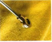
er local parts stores. Solder the tubing in place. After allowing to cool, bend and cut the new tubes to fit your car. Most brake tubing can be bent without a tubing bender. But be careful
