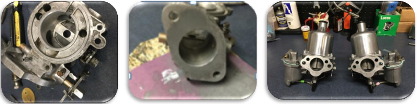
Figure 4. Filing the Idle Screw Divot; Sanding Flanges Flat; and the Finished Product
