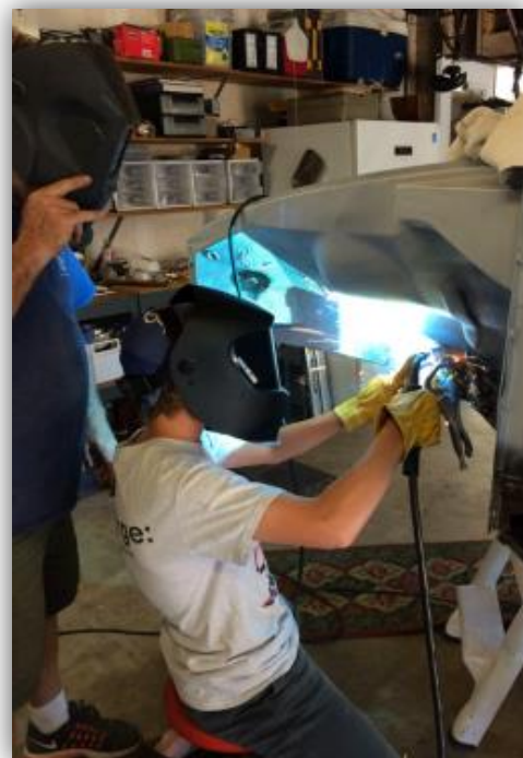
Joseph welding up the frame rail.
