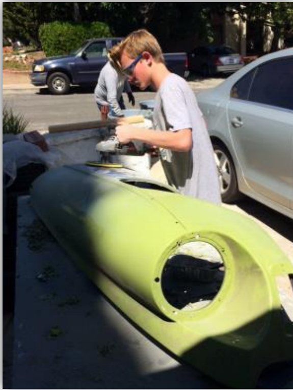
Grinding off the old paint
