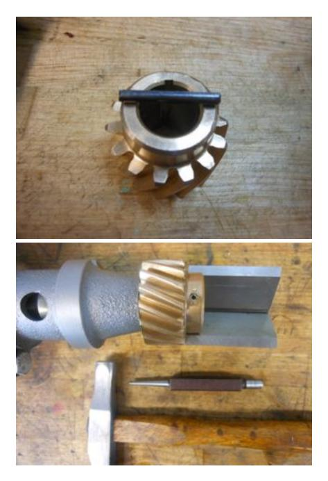
Note: it is somewhat maddening that new drive gears have the pin bores predrilled. This is unnecessary and requires additional effort to accurately
