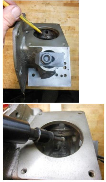
2. As water enters the pump, it must negotiate an abrupt transition to the vane cavity. This can be enhanced by tapering the entrance. The coolant is subjected to less turbulence and flow is enhanced.
