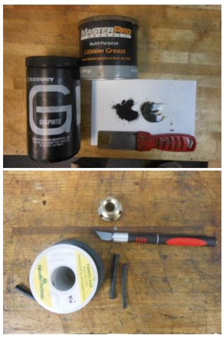
4. To facilitate the assembly of the pump shaft through the packing installed in the pump, a shaft of the same diameter as the pump shaft (.500") can be installed while installing the packing and a machined tube slid over the shaft
