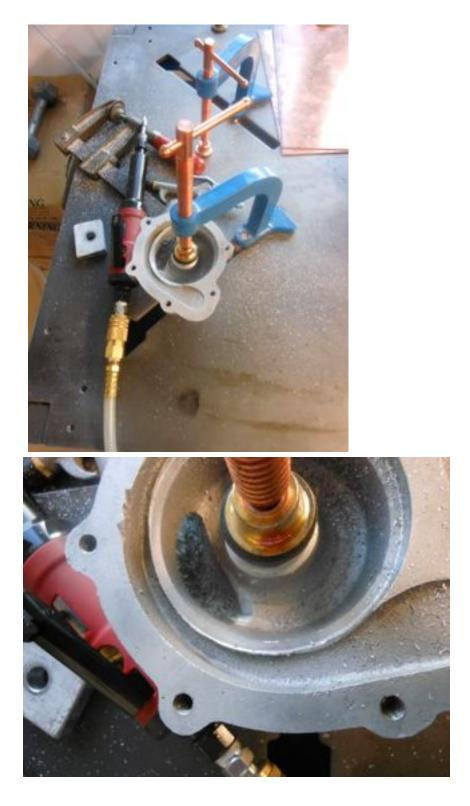
3. For many years, I used 1/8" water pump packing and wound it around the shaft (opposite to rotation) and enhanced its lubrication with Penrite water pump grease laced with graphite powder. Today, an acceptable variation is to
