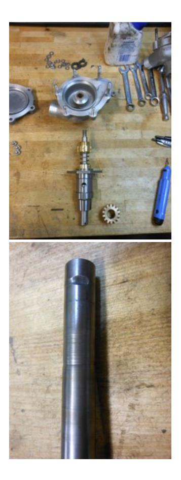
If one disassembles their pump and elects to convert to a high volume impeller as described, be forewarned that the job is not easily accomplished and requires some machine setups to modify the castings. The impeller bores in the pump lids will need to be machined deeper as well as a similar treatment to the pump bodies. In addition, a modification to the center casting to accept the impeller vanes will need to be accomplished.
