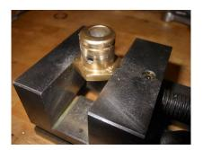
The remedy is to grasp the rocker in a suitable vice and with a round or half round diamond file, dress this edge so that a chamfer is created on the inside paring line.
