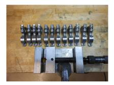
Two additional operations help secure rocker arm success. Dress the sharp edges with a Cratex or felt grit- impregnated wheel and then sonic clean the rockers followed by swabbing with a miniature brush. Inspect with a pin light.
