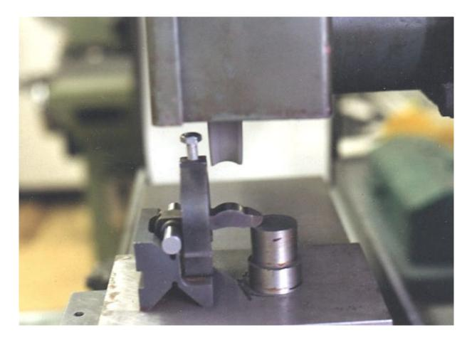
One remedy is to carefully dress each surface with the Arkansas stone and then polish with emory on a buffing wheel. The result will yield an array of surfaces that shine like a mirror and result in much reduced abrasion both to the cam lobes and valve stem ends.
