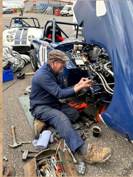
The paddock was busy with through the weekend with repairs and adjustments. John Hughes had a failure in Race 1 with o/s front axle bearing which had welded itself to the stub axle. Richard Perry came to the rescue with a replacement which the Hughes talented spanner man Ian Blaine(see above) fixed for second race.
