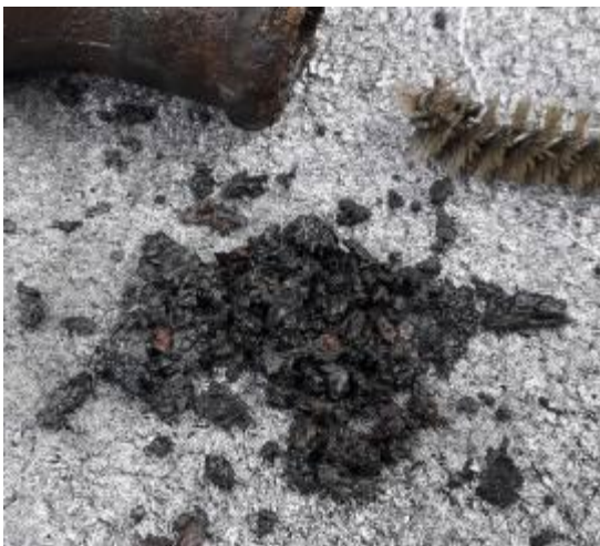
Photo 3 – General Cooling Crud
