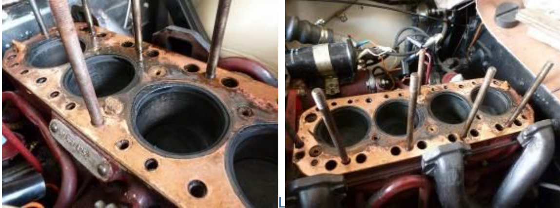
Joe's cylinder block, with blocked waterways and leakage patterns
