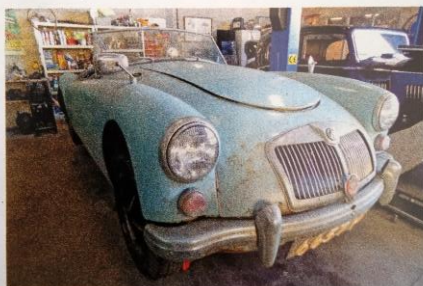
The MGAs wings are now made from glassfibre, says Chris McPheat, who is restoring it
