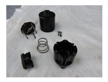
8. To remove the old piston seal it is necessary to drill out the centre rivet which passes through the large washer, the leather seal, piston and is swaged over on the inner piston face.
