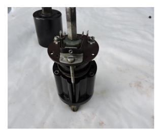
7. Remove the contact plate, piston and spring
