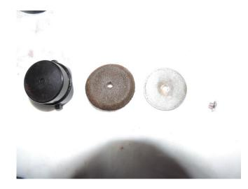
9. Clean all parts as necessary ensuring old grease is removed.10. Inspect the switch contacts which should be silver tip. If pitted polish
