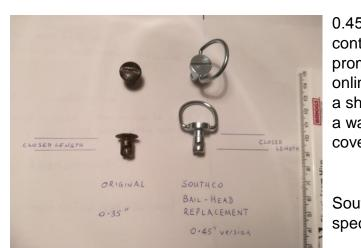
**45** is 0.45" the CLOSED length of the fastening, the distance from underside of head to the top of the slot.
