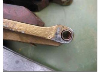
The copper sleeves now take on the role of the sacrificial wearing part and can simply be replaced when needed. This, along with new, lightly greased bolts has the carriers nice and snug, they can rotate and there is no top fore and aft sway at all.
