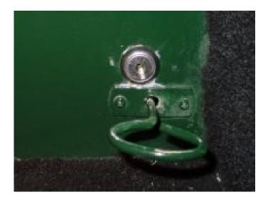
The lock lever is then notched to fit around the operating rod and the U clamp (6mm internal diameter) bolted in place to prevent the boot from opening. The exact positioning of the clamp is by trial and error.
