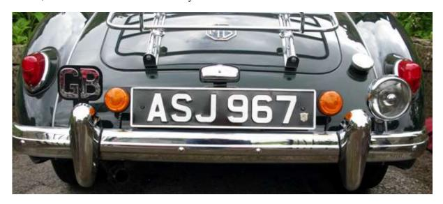
Here are other examples of orange rear lamps fitted to 1500 MGAs
